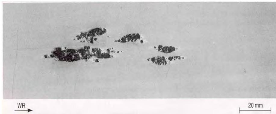
**Figure 2:** Surface defect "Sticky Scale" (Rolled in primary scale) [2]
