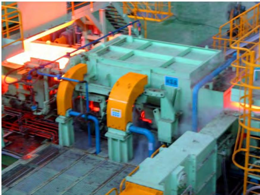
**Figure 11:** View of the descaler at the entry of the finishing mill of the Hyundai Steel hot strip mill
