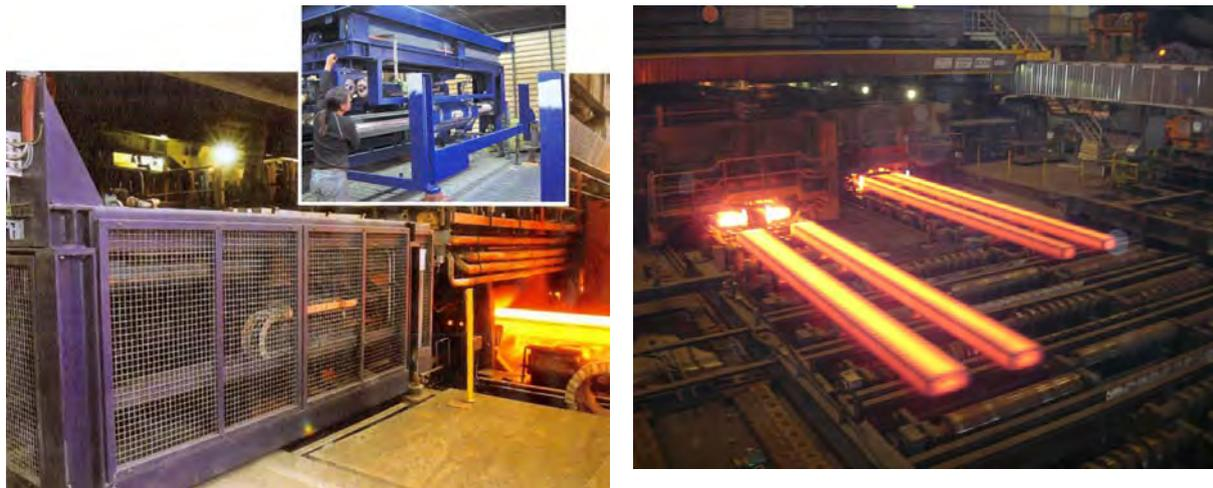
**Figure 12:** Descaling system for the slab casting plant with four individual strands at HKM
